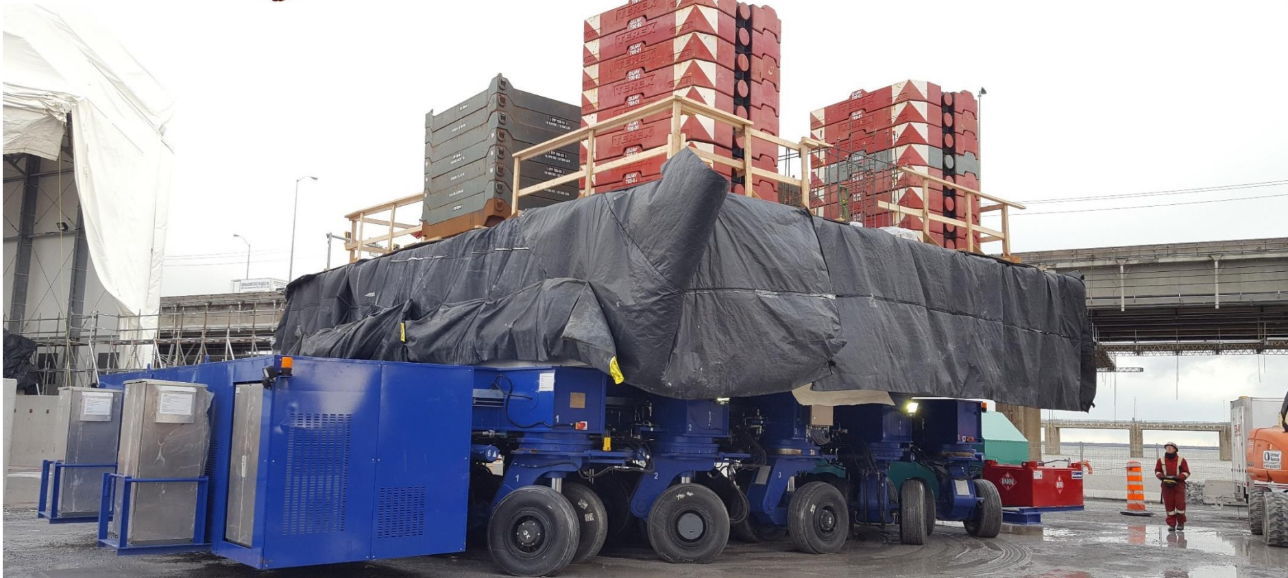
1000 tonne capacity Transporter, New Champlain Bridge, Canada
