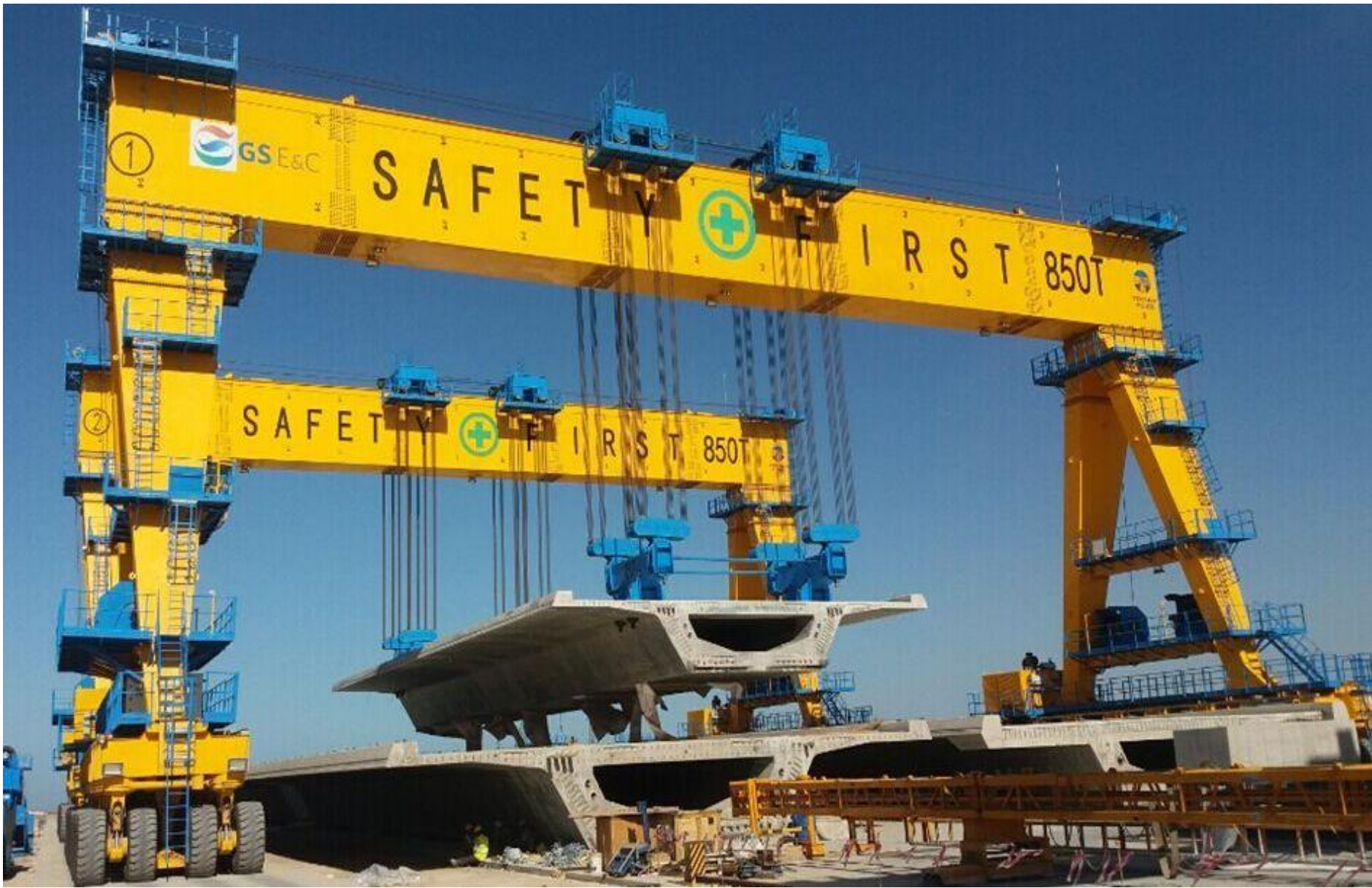
Doha Link straddle carrier, 2 x 850 tonne capacity, Kuwait
